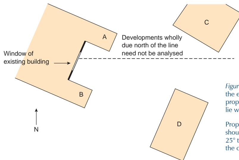
Figure 27: In analysing the sunlighting impact on the existing window, no check need be made for proposed extension A and new building C, as they lie within 90° of due north of the window.
