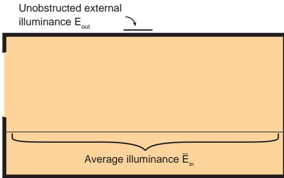
Figure 5: Definition of ADF. Under standard overcast conditions:
