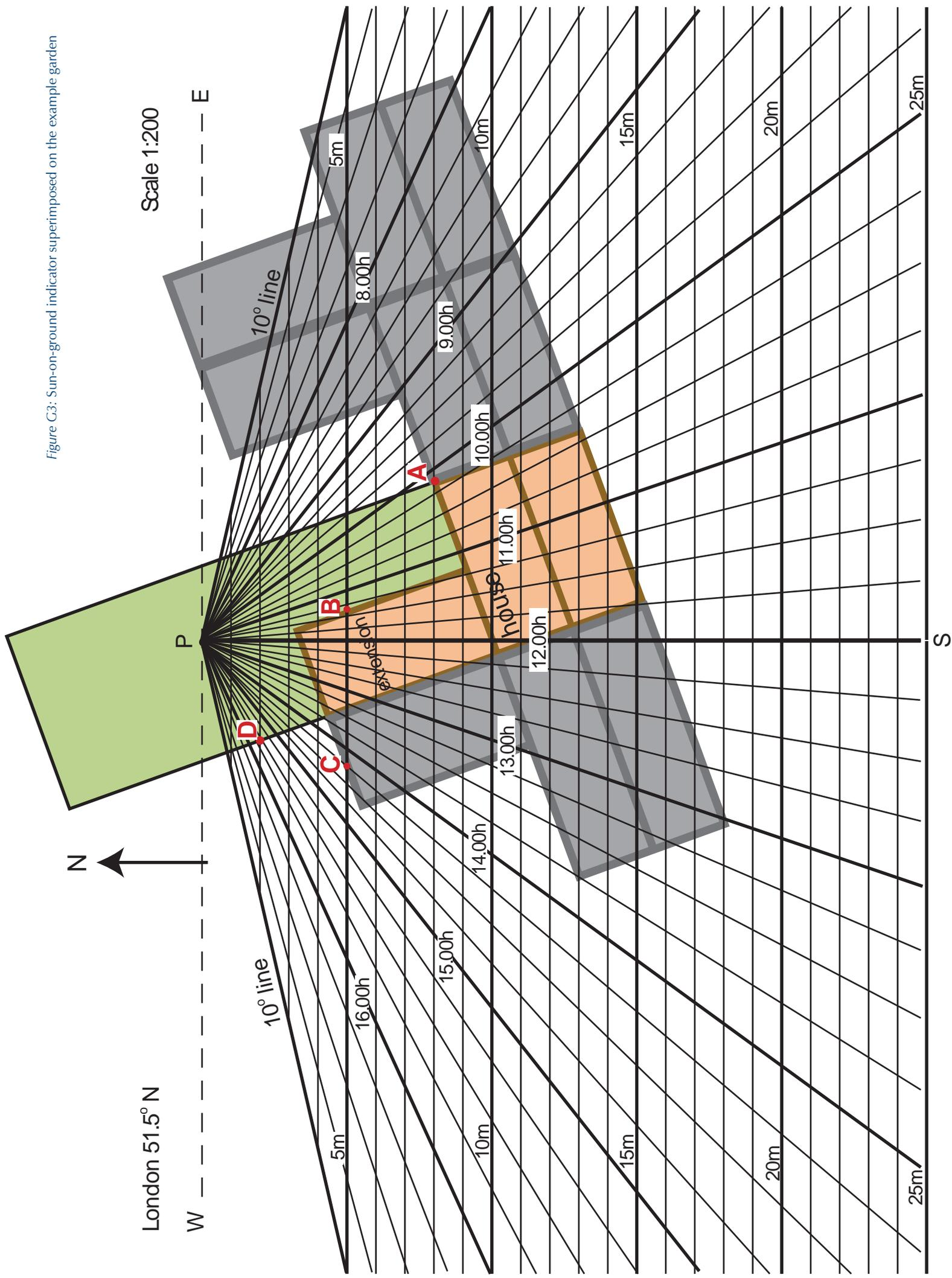
G6 The horizontal lines running across the indicator give the height of obstructions which would just stop the sun from shining on point P at each time of day. These heights are relative to the point on the ground. On sloping ground, take care that the height used is the actual height of the top of the obstruction above the particular reference point.
