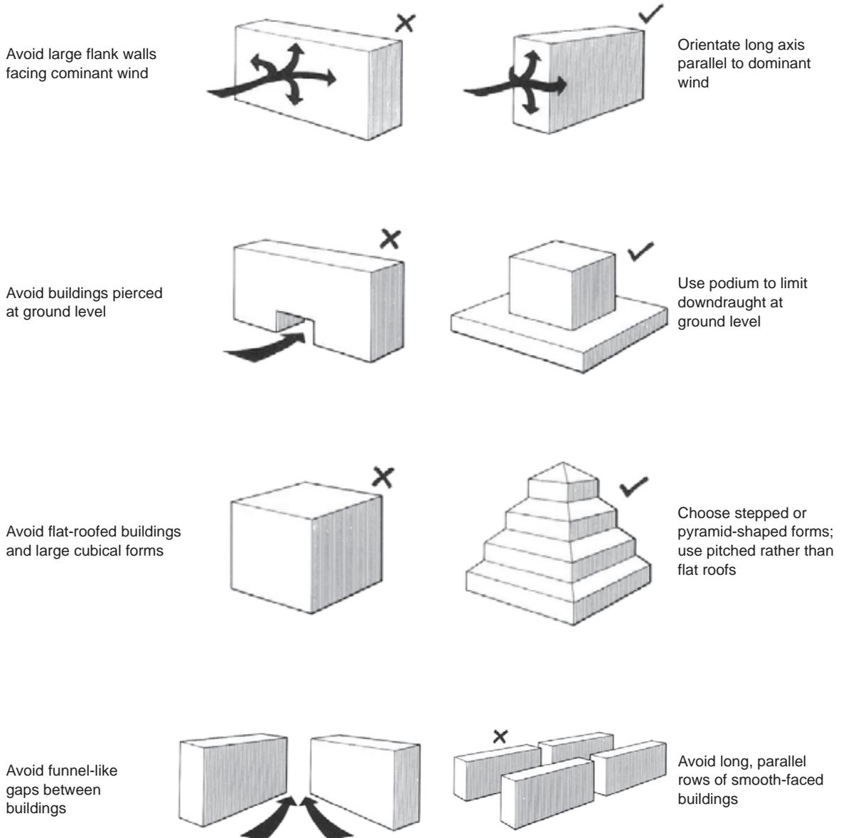
Figure 38: Reducing the wind sensitivity of buildings
